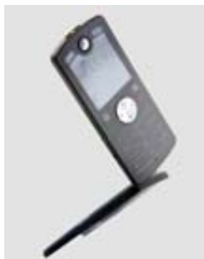
The Group's bistable display IC supported Motorola's Motofone, the world's first mobile phone with E-paper display.
